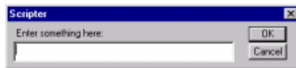
Example of the InputBox function. The text entered in the box is returned to the script.
