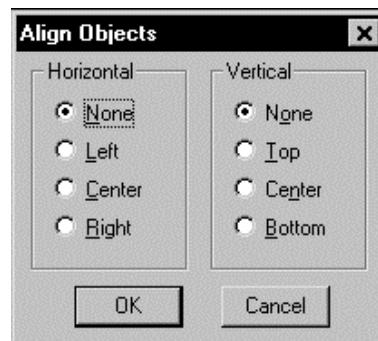
The Align Objects dialog box shows the Horizontal and Vertical alignment for the selected objects.
